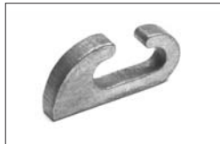
H-2 Hook Part No. 44102-11 Flame-cut from 5/8-in. material and can be welded flat on trucks. Accepts web loops, D-rings, cable or rope. Meets CHP anchorage requirements when properly secured. Weight: .61 lb./ .28 kg.
